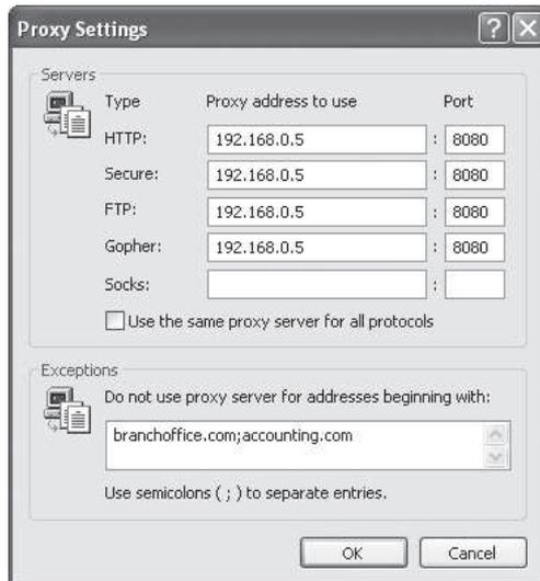
**Figure 7-12** Example Nontransparent Proxy Configuration
