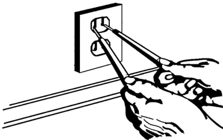
**1-4** Checking voltage at a 125-VAC duplex receptacle.
