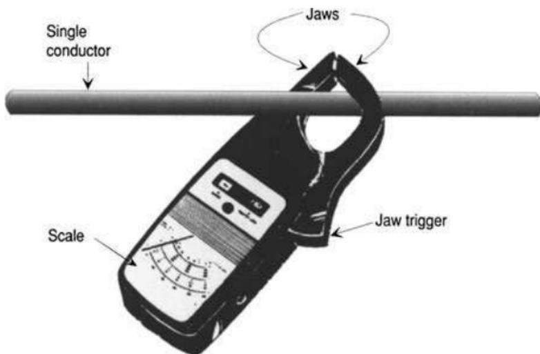
**1-1** Typical clamp-on-type ammeter.
