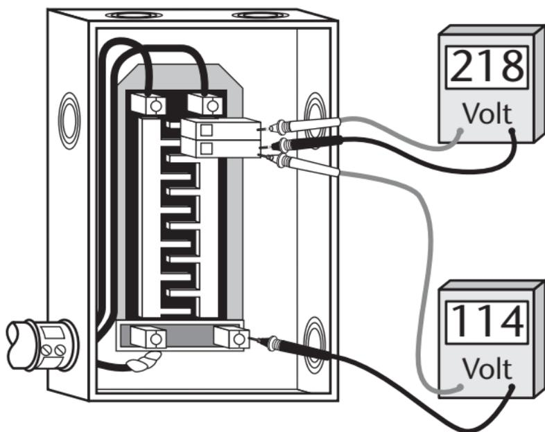
**9-4 Safe voltage measurement technique at panel board.**
