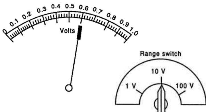
To find the voltage across a component, multiply the scale reading by the setting of the range switch:
