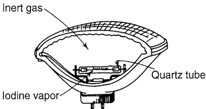
5-3 Basic components of a tungsten-halogen lamp.
