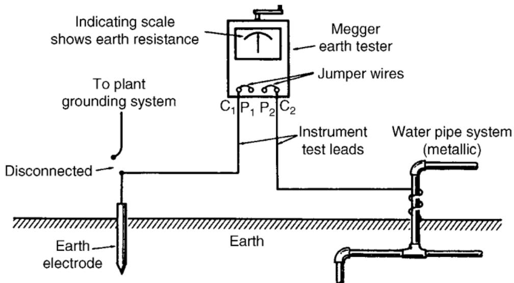
**1-13** Direct method of earth-resistance testing.
