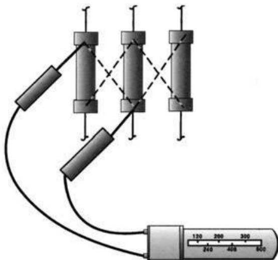
**1-8** Testing fuses with a voltmeter.
