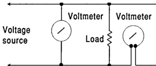
**1-3** Connecting a voltmeter to a circuit.
