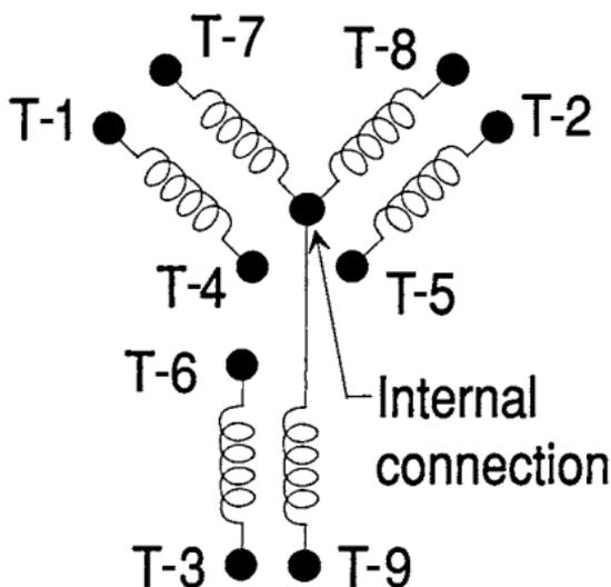
**6-4 Simplified electrical arrangement of wye-wound motor coils.**
