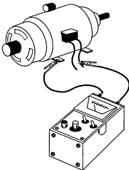
**1-12** Method of testing an AC motor.
