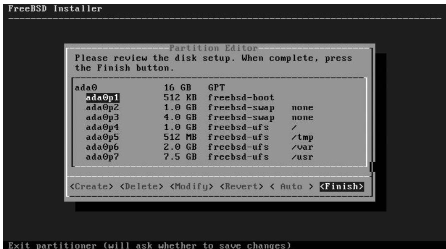
Figure 3-14: Complete custom GPT/UFS partition table
