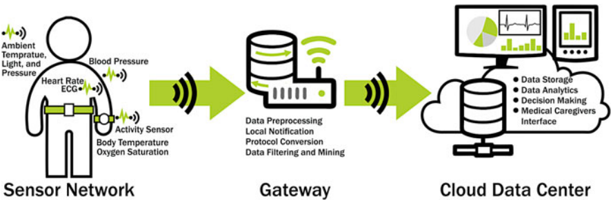
Fig. 8.4 Healthcare IoT system architecture
